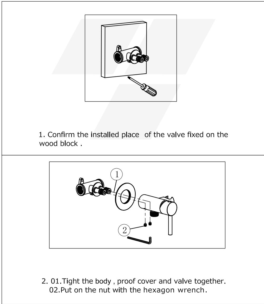
1. Confirm the installed place of the valve fixed on the wood block .
