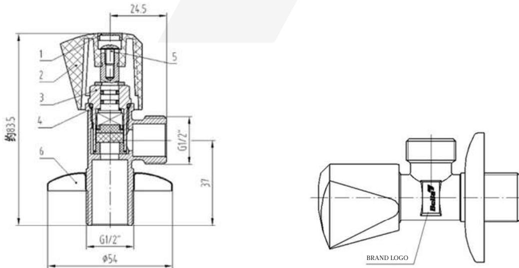
1. The O ring and the spool connection thread are coated with silicone grease to ensure lubrication.
